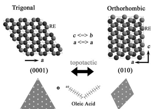
Scheme 2. Crystal structures of trigonal \text{REF}_3 viewed along the (0001) crystal plane and orthorhombic \text{REF}_3 viewed along the (010) crystal plane (the direction perpendicular to the nanoplates); the schematic arrangement of rare-earth cations and oleic acid ligands on the nanoplates. Oleic acid is assumed to be attached to the surface \text{RE}^{3+} ions.
